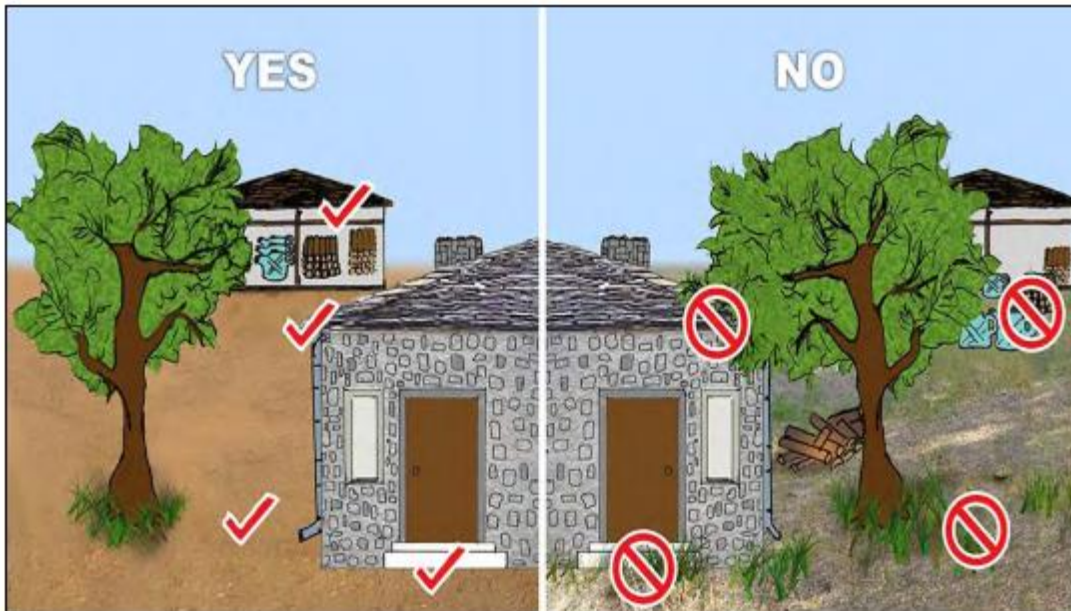
Figure 6. Removing the living and dead vegetation and firewood storage nearby houses and outbuildings is needed to make them safer upon wildfires [32]
