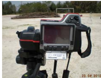
Thermographic camera in the field (FLIR P65)
