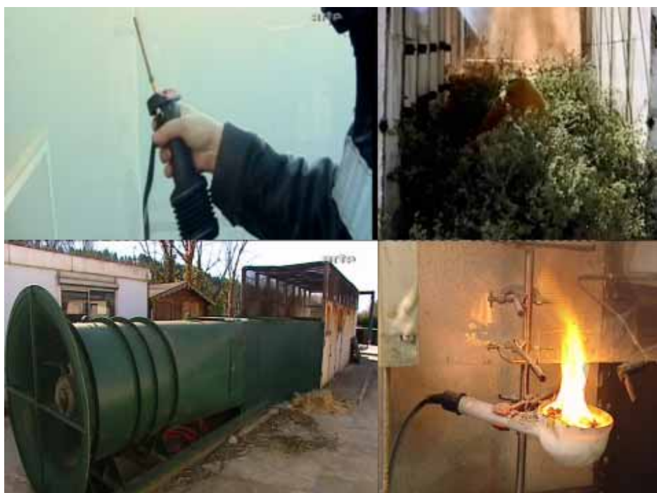
Figure 4. Smoke sampling in fire tunnels and in the laboratory.
