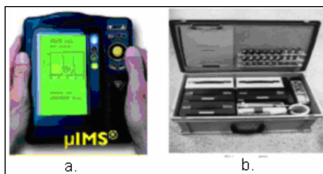
Figure 4. Miniaturized IMS (a) and a Hand-held field luggage (b).
