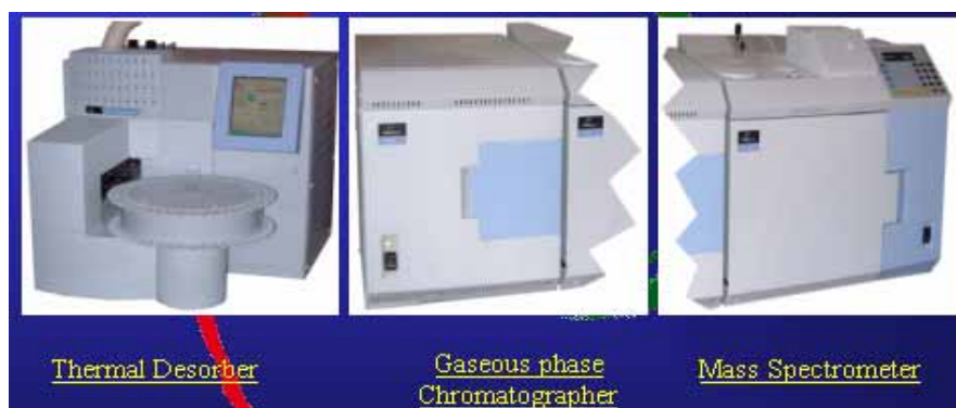
Figure 2. Thermal desorber, Gaseous phase Chromatographer and Mass Spectrometer Turbo Mass Gold (Perkin Elmer).
