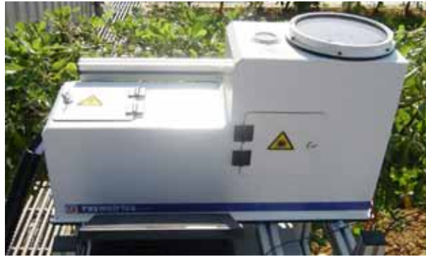
Figure 2. The Raymetrics LB11 LIDAR system designed and developed to perform continuous measurements of the suspended aerosols particles in the PBL and the lower free troposphere.
