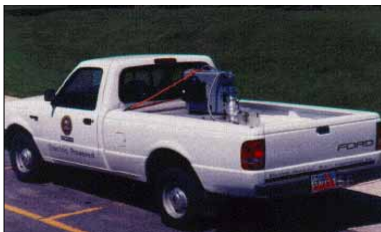
Figure 3. Roving GC/MS instrument mounted on the bed of an electric-powered truck.
