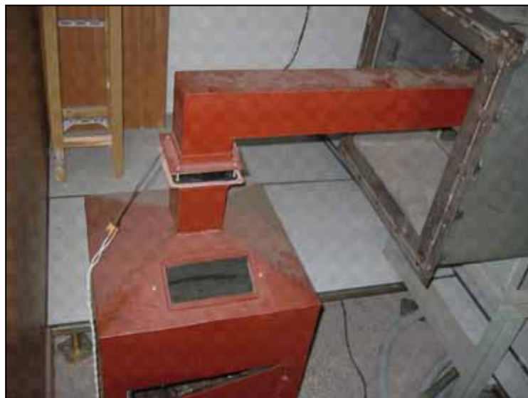
Figure 4. 60 smoldering cottons put in the smoke-generating box.
