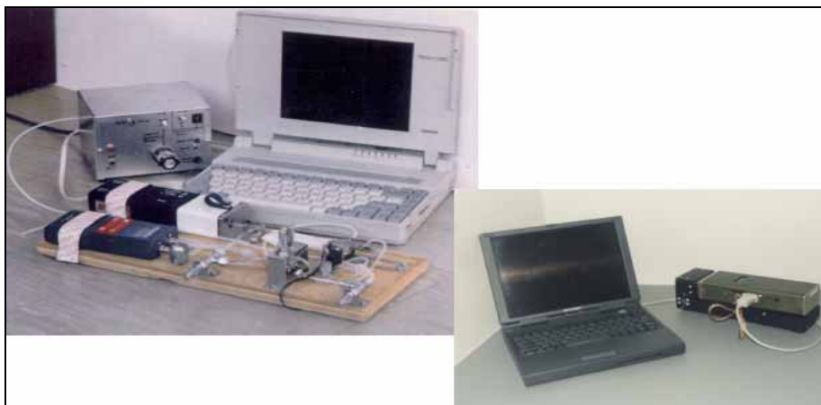
Figure 12. Breadboard Hand-portable AVS-TLGC/IMS instrument (Prototype).
