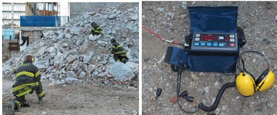
Figure 2. Many rescue/USAR teams use a sound magnifier to detect the victim’s voice under the ruins
