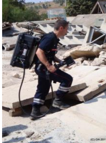
Figure 3. Device for location of entrapped people, which provides with chemical “Life Signs” along with audio and visual data (FIRST device)[30]
