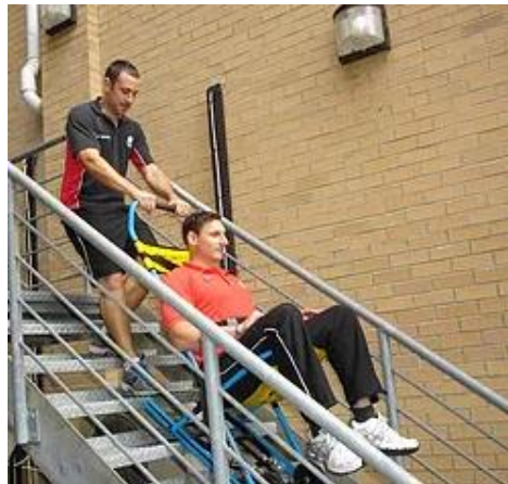
Figure 12. Evacuation chair used for evacuation of mobility impaired people (Red Hawk Training http://www.redhawktraining.com/single-post/2014/08/25/New-Evacuation-Chair-Training-Course ) [49]
