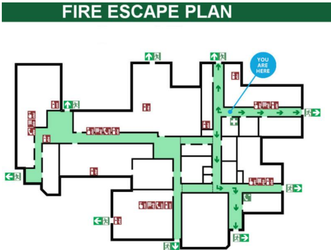
Figure 5. Indicative “Fire Escape Plan” according to ISO 23601:2009 [39]
